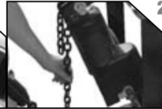
2. Push lift arm down until there is a little slack in the chain.
