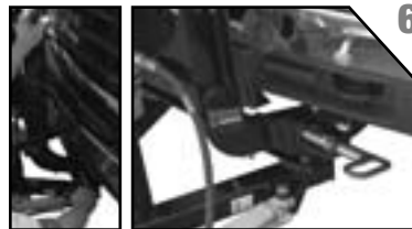
6. While slightly pushing the lift frame towards vehicle, pull handles on either side to disengage pins then twist until the leg locks the pin in the open position.
