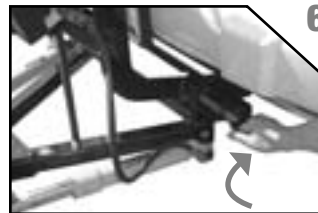
6. Pull handle on driver's side to disengage pins then twist until the notch locks the pins in the open position.
