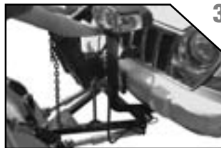
3. Push back on lift frame until pins spring thru mount on vehicle.
