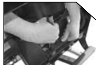
4. Press down jackstand lever and lower jackstand to ground, then release lever.
