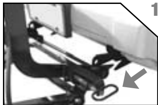
1. Pull vehicle into plow assembly and push plow assembly forward an inch or two.
