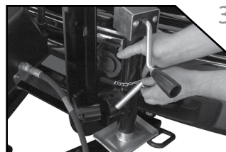
3. Remove crankstand from lift frame.
