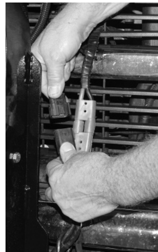
All electrical connections cleaned and add dielectric grease once/month
