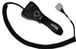
light indicates the snow plow is now in the Lower/Float position. In this position the snow plow will be able to follow the contour of the road and the snow plow can also be angled to the left or right. Touching the up arrow automatically cancels the Lower/Float position.
