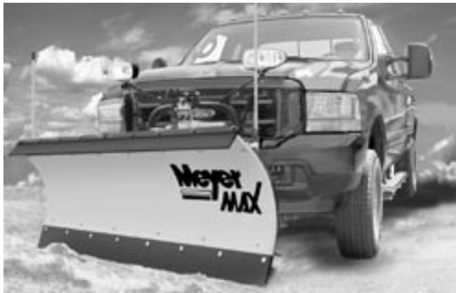
plow path, in the angled position, should exceed the tire track by at least six inches on either side. Be sure to have enough slack in the lift chain while plowing so the cutting edge of the moldboard can follow the ground contour. Use the adjustable runner shoes to set the bottom edge of the plow just above the ground for best operation.
