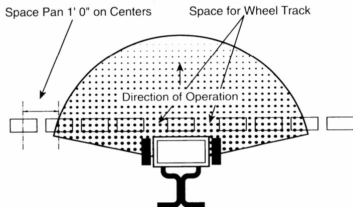
effective pattern width is the distance out from the spreader to a point where the amount of material is 1/2 the average amount in the center pans. This distance is multiplied by 2 to achieve the total effective pattern width.
