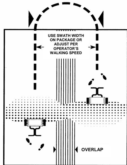
**6.** Push spreader at a normal walking speed - 2 1/2 m.p.h. (18 feet in 5 seconds). Apply header strips around area to be treated. Space trips across the area as shown. Keep material off flower beds, sidewalks, etc.
