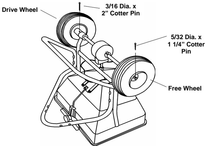
**2.** Slide drive and free wheel onto axle as shown with the longer portion of wheel hub facing the frame. Secure free wheel with (1) 5/32 dia. x 1 1/4" cotter pin. Attach drive wheel to axle with (1) 3/16 dia. x 2" cotter pin.
