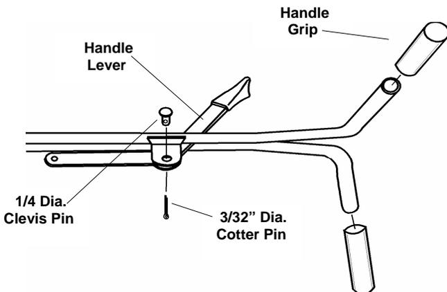
**4.** Slide handle lever between handle brackets as shown and secure with (1) 1/4 dia. clevis pin and 3/32" dia. cotter pin. Make sure lever pivots freely. Install handle grips onto upper handle.
