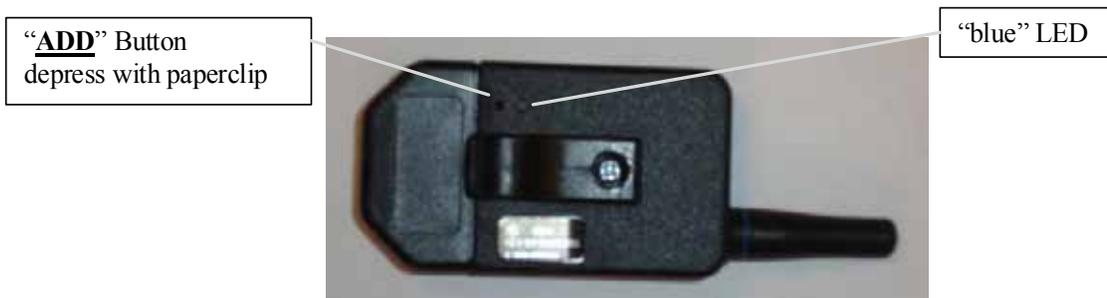
**Fig. 2: Transmitter Back Button Assignments**
