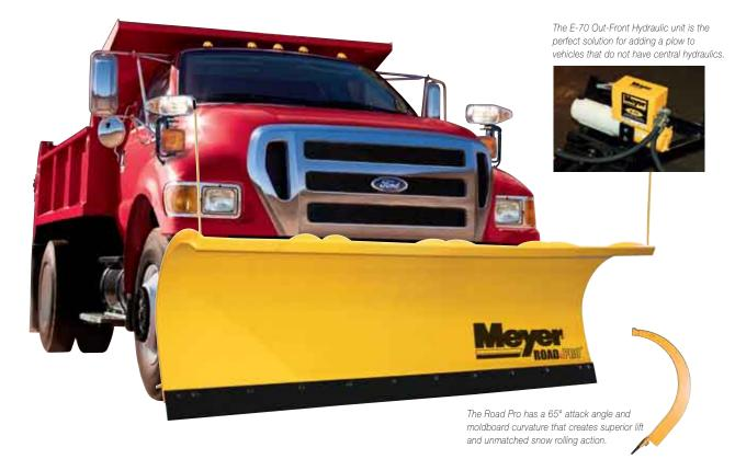
HM WORKS WITH: 17,000-26,000 GVW MOUNTING SYSTEM: Universal OPERATING SYSTEM: E-70 or Central Hydraulics ROAD PRO WORKS WITH: 26,000-33,000 GVW MOUNTING SYSTEM: Universal OPERATING SYSTEM: Uses vehicle central hydraulic system
