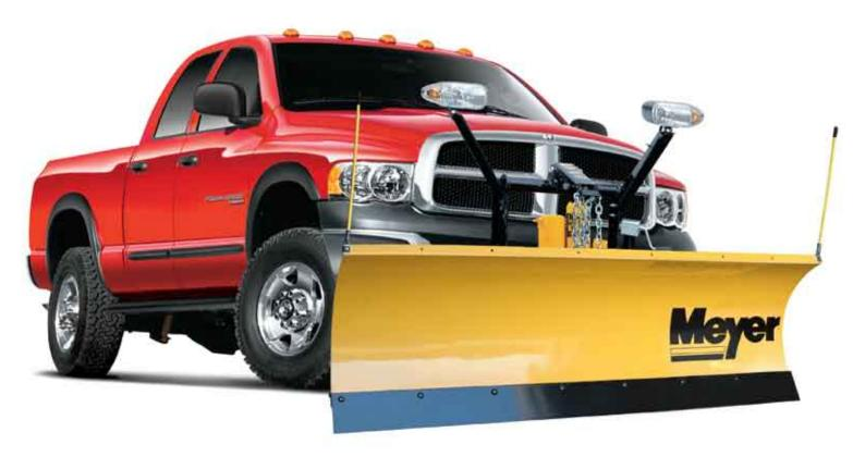
WORKS WITH: 3/4 ton and up MOUNTING SYSTEM: EZ-Mount Plus OPERATING SYSTEM: E-58H
