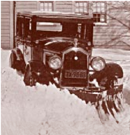
When the snow is blocking the road, Edward B. Meyer of Downing Avenue does not lay up his car or wait for the Public Service plows to make a path. He hooks up a plow of his own device to his Buick and away he goes. With J.A. Davis, local photographer, he recently ran up the plow in five minutes. It is made of light iron, fashioned by Mr. Wents of the Newburgh Iron Works.
