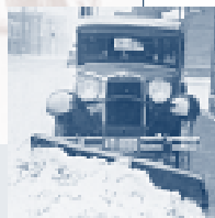
► 1930 The 1930's Black Hawk Jack operated by a starter motor; the first electric hydraulic lift later modified to become the Meyer T-1 Electric Hydraulic lift.
