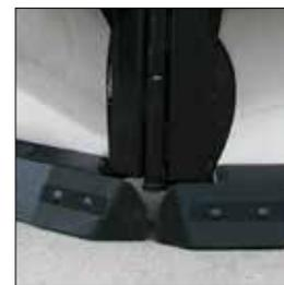
A direct replacement for standard rubber center kits, the Super-V/V<sup>2</sup> urethane center kit provides clean clearing performance without adjustment and will not mar the surface. One kit fits all Super-V/V<sup>2</sup> plows. #08409
