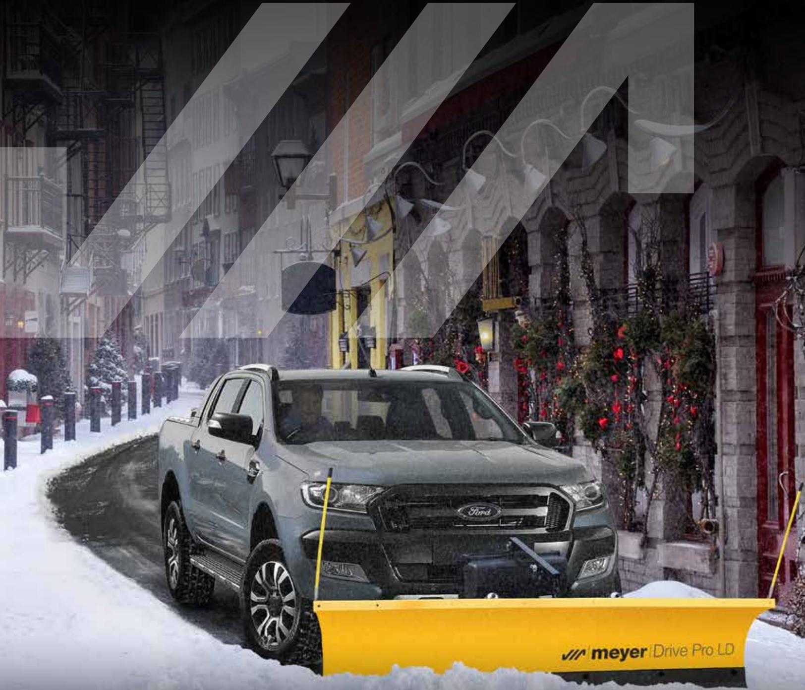
When you add a Meyer® Drive Pro LD to your SUV or light truck, you get the perfect solution for plowing small lots, long driveways or any narrow area where a large truck can't fit. This lightweight contractor-grade steel plow features a 5cm receiver mount and 2,03m moldboard. The Drive Pro LD is available with full hydraulics for up/down/left/right plow movement.
