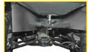
Impeller spinner shaft adjusts the spread pattern from 3'-4' to 8'-10'.
