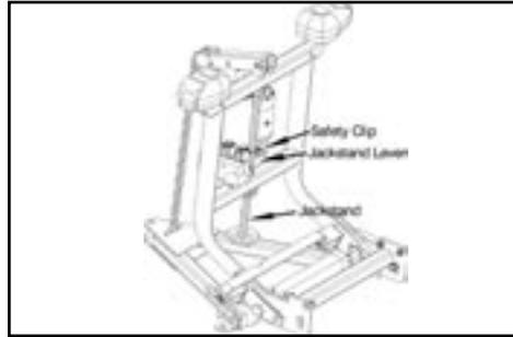
**2** Remove Safety Clip from jackstand. Push Jackstand Lever down to lower Jackstand to ground. At the same time, push lift frame up and toward the vehicle. Reinstall Safety Clip to Jackstand below the lift frame.
