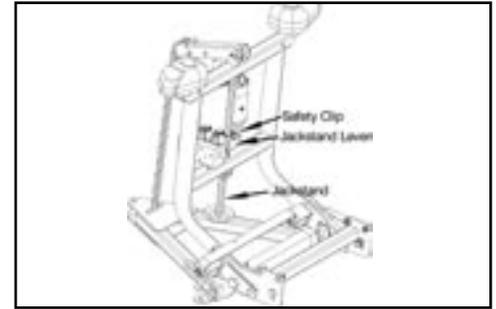
**3** Remove Safety Clip from jackstand. Push Jackstand Lever down and raise Jackstand to storage position. Reinstall Safety Clip to Jackstand above the lift frame.
