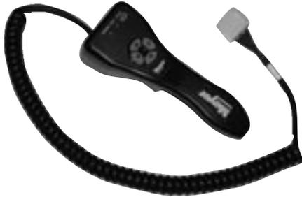
light indicates the snow plow is now in the Lower/Float position. In this position the snow plow will be able to follow the contour of the road and the snow plow can also be angled to the left or right. Touching the up arrow automatically cancels the Lower/Float position.
