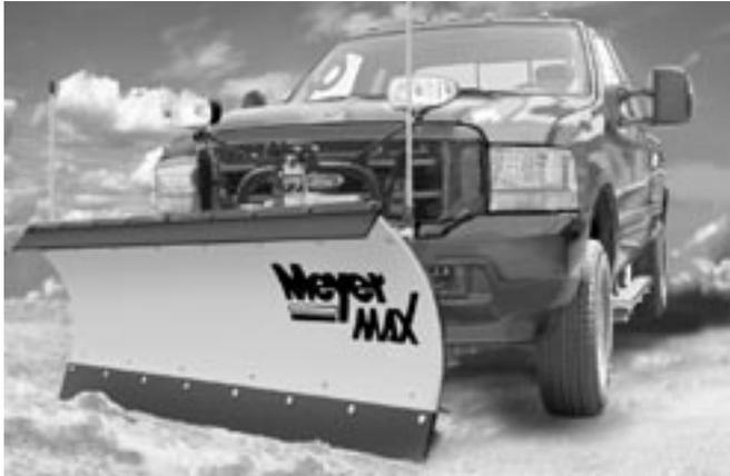
plow path, in the angled position, should exceed the tire track by at least two inches on either side. Be sure to have enough slack in the lift chain while plowing so the cutting edge of the moldboard can follow the ground contour. Use the adjustable runner shoes to set the bottom edge of the plow just above the ground for best operation.
