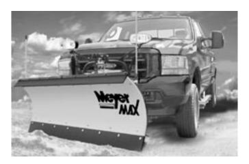
plow path, in the angled position, should exceed the tire track by at least two inches on either side. Be sure to have enough slack in the lift chain while plowing so the cutting edge of the moldboard can follow the ground contour. Use the adjustable runner shoes to set the bottom edge of the plow just above the ground for best operation.
