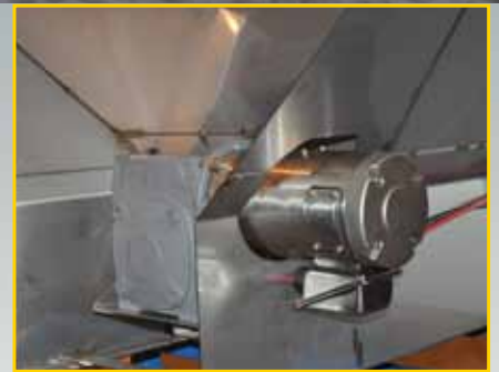
Auger and spinner are driven independently by two electric motors.
