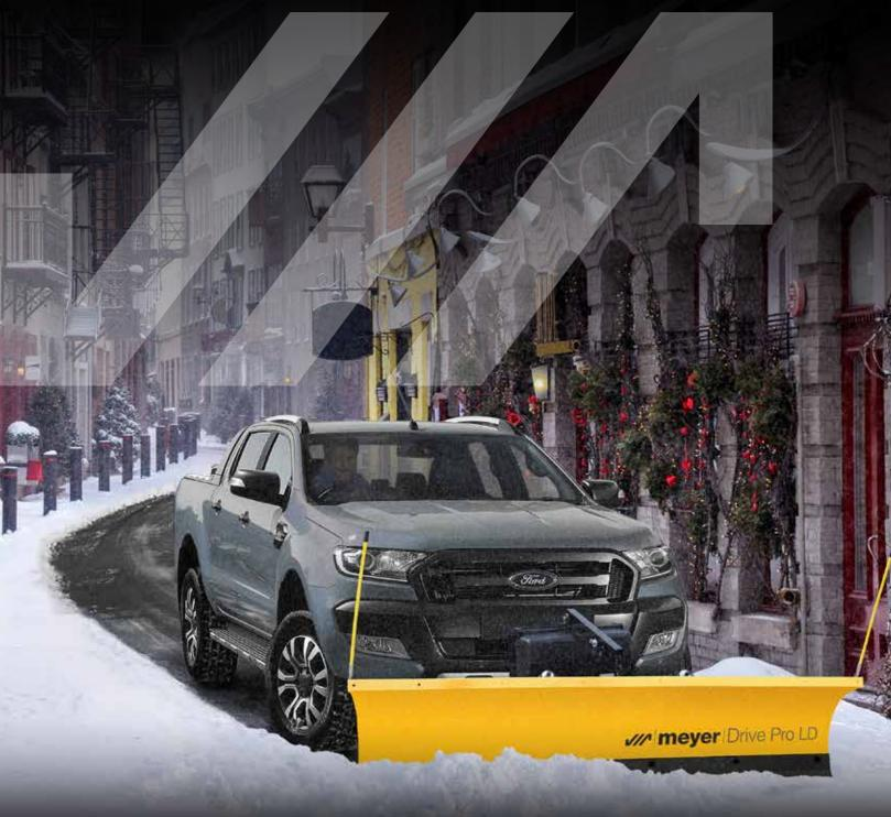
When you add a Meyer® Drive Pro LD to your SUV or light truck, you get the perfect solution for plowing small lots, long driveways or any narrow area where a large truck can't fit. This lightweight contractor-grade steel plow features a 5cm receiver mount and 2,03m moldboard. The Drive Pro LD is available with full hydraulics for up/down/left/right plow movement.
